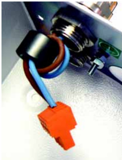
Figure 1-5. Looping Relays Connection Wires Around a Suppression Ferrite
