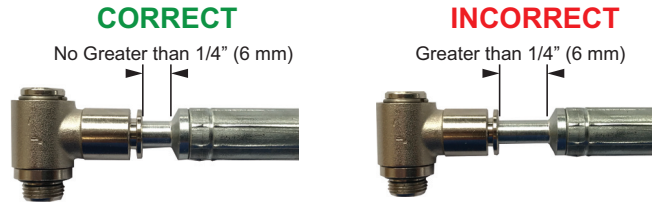
Figure 4-16. Actuation Hose Install
