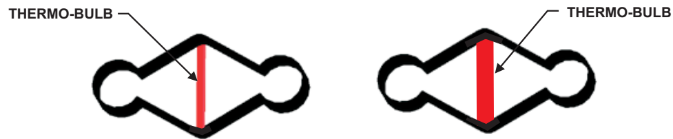
Figure 2-22. Thermo-Bulb Link, P/N 87-12009X-XXX
