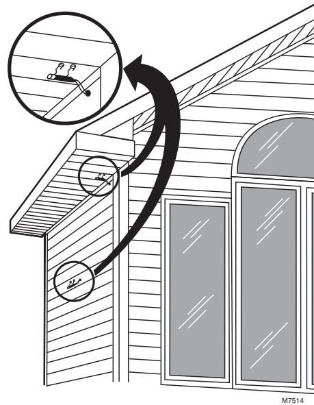
Fig. 69. Typical locations for C7089U1006 Outdoor Sensor.
