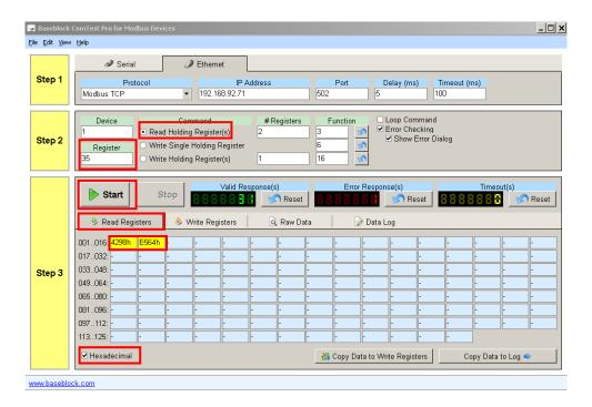
Record the register readings and plug them in the IEEE calculator. As this value is a Hexadecimal value, select the "Hex" option radial button in the calculator.
