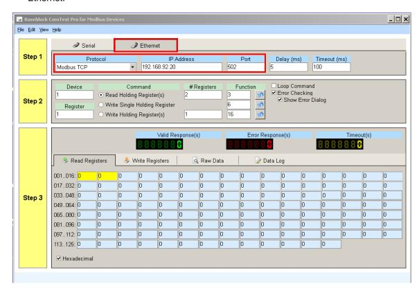
In the initial test we will change the burner set-point from its current value to 150F. If the current value is already 150F, select another set-point value to insure Modbus communication is functioning.
