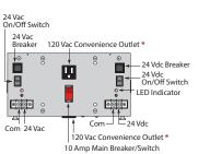
Move internal jumper to "HOT" position if you wish outlets to always be hot otherwise outlets will be switched by main breaker.
