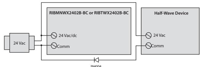
^^ Option 2: Add diode on 24 Vac power (Comm) interconnection between devices. Band on diode faces towards RIB(s).
