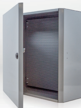
NEMA 1, 16 Gauge 18" x 18" x 7" Key Latch Door MH4404L shown w/ perforated steel sub-panel
