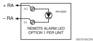
Note: Remove jumper when using RA100ZA with the intelligent duct smoke detector.
