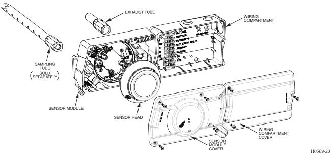
NOTE: Sensor Module sold separately. Refer to the control panel technical documentation for compatible ULC-listed heads with Remote Test Capability.
