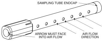
CAUTION: The sampling tube end cap, included with the detector, is critical to proper operation of the duct smoke detector. The end cap is needed to create the proper air flow to the sensor of the duct smoke detector. Once any sampling tube length adjustments are made, plug the end of the sampling tube with the provided end cap.
