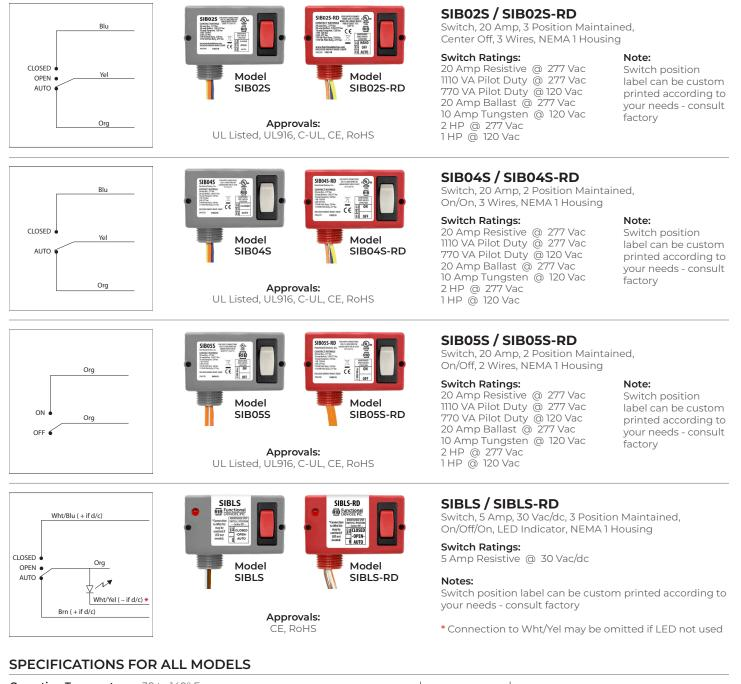
Operating Temperature: -30 to 140° F Humidity Range: 5 to 95% (noncondensing) Origin: Made of US and non-US parts Wires: 16", 600V Rated Housing Rating: UL Accepted for Use in Plenum, NEMA 1
