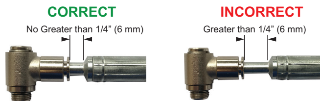
Figure 7-1. Actuation Hose Install
