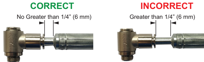
Figure 4-18. Actuation Hose Install
