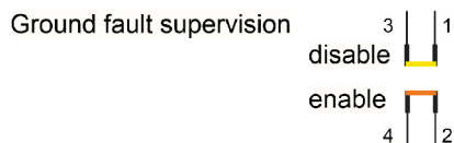
Figure 2 Ground fault detection jumper settings
