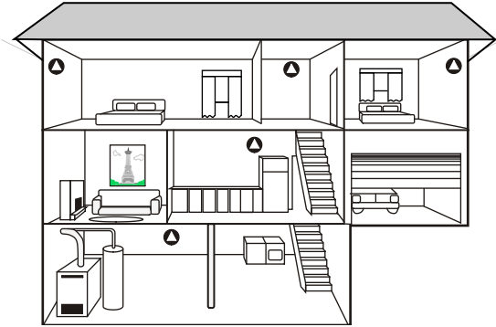
Figure 1: Recommended CO detector locations
